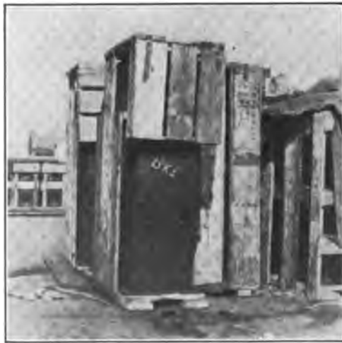
FIG. 140.—Blower crated for export; note crating over pulley and outboard bearing.
